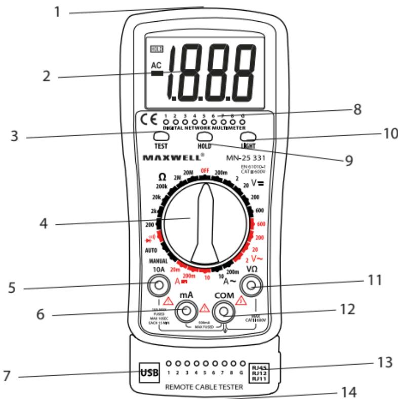
1. RJ45, RJ11, RJ12, USB test connector
