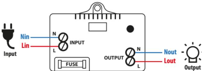
Connect the disconnected mains lead to the sockets marked "INPUT".
